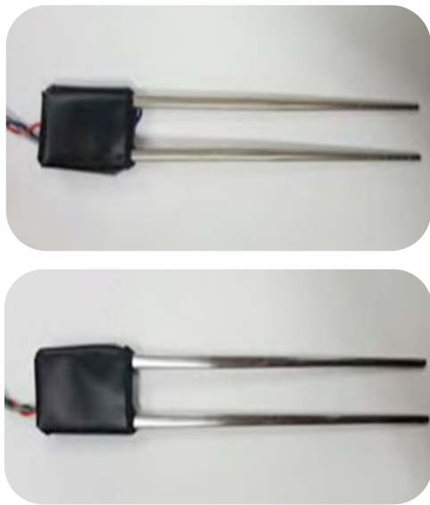
Fig. 8. Developed Soil Humidity Sensor (Vacuum chopsticks on the top, stainless chopsticks on the bottom)
