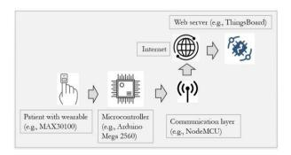
Fig. 4: The block diagram of a remote health monitoring system
