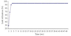
Fig. 6: Link utilization for bottleneck link with five flows
