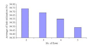
Fig. 7: Average of link utilization for bottleneck link with different numbers of flows
