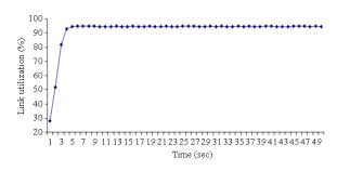
Fig. 4: Link utilization for bottleneck link with three flows
