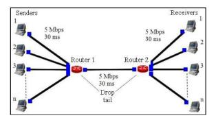
Fig. 2: Multiple flow experimental set-up for New-AIMD evaluation
