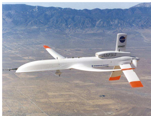
Fig. 10. ERAST is a multiyear effort to develop the aeronautical and sensor technologies for a new family of remotely piloted aircraft intended for upper atmospheric science missions. Source: Petrescu and Petrescu (2011)
