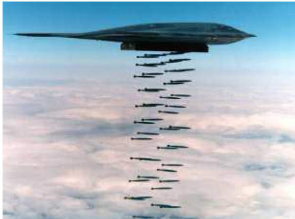
Fig. 16. In a 1994 live fire exercise near Point Mugu, California, a B-2 drops 47 500 lb (230 kg) class Mark 82 bombs, which is more than half of a B-2's total ordnance payload. Source: (Petrescu and Petrescu, 2013b)
