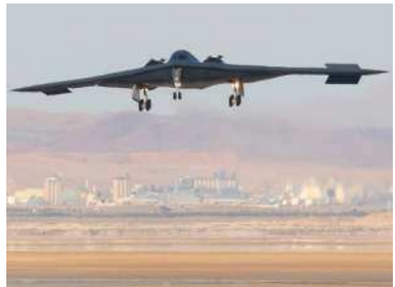
Fig. 24. Flying wings are very efficient aerodynamically, with much less drag than ordinary aircraft. Source: (Petrescu and Petrescu, 2013b)
