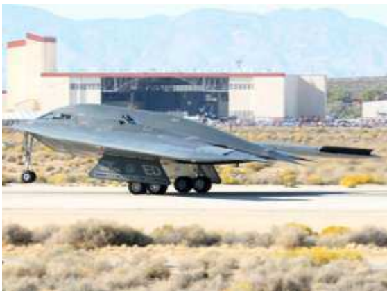
Fig. 21. The unusual scoops on top of the engine pods are auxiliary air intakes which are needed to get extra air flow into the engines at low speeds. Source: (Petrescu and Petrescu, 2013b)
