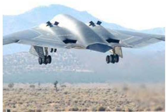
Fig. 23. The four non-afterburning engines are buried within the wing. Source: (Petrescu and Petrescu, 2013b)
