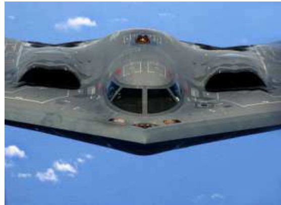
Fig. 14. The B-2's engines are buried within its wing to conceal the engines' fans and minimize their exhaust signature. Source: (Petrescu and Petrescu, 2013b)
