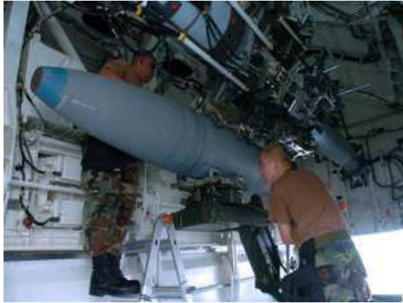
Fig. 12. A 2000 lb BDU-56 bomb is being loaded onto a bomb bays rotary launcher, 2004 Source: (Petrescu and Petrescu, 2013b)
