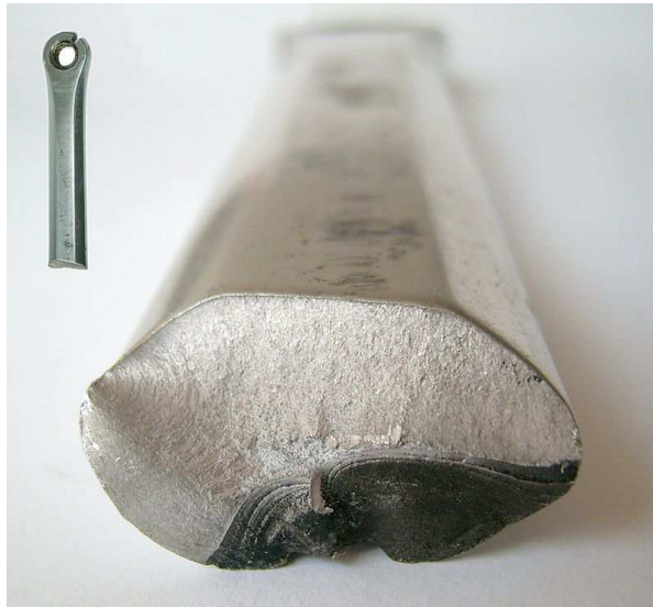
Fig. 8. Fatigue (crank of bike crank): we can distinguish the lines of progression of cracks in the bottom right (dark zone), and the zone of removal (clear zone)
