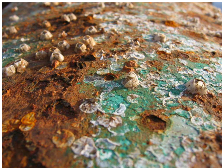
Fig. 16. Antifoulings only temporarily limit the corrosion of boat hulls
