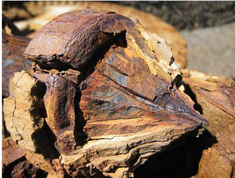
Fig. 17. A mine machine abandoned in a mine. The corrosion of the steel can be exacerbated by moist air, or here acidified by vapors of volcanic origin
