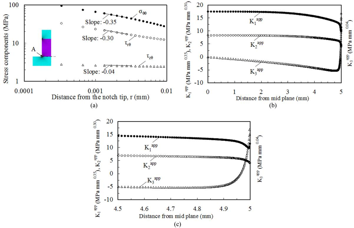
Fig. 2. Stress components along the adhesion line, as a function of the distance from point A, at the distance  $z = 0.5$  mm from the lateral free surface of the joint (a); plots of the apparent NSIFs along the width of the joint (b) and in the vicinity of the lateral surface,  $4.5 \leq z \leq 5.0$  mm, (c)
