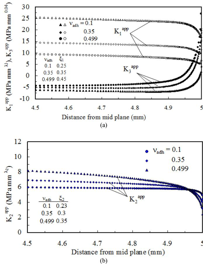
Fig. 4. Plots of the A-NSIFs along the width of the joint, at the lower interface, for different Poisson's ratio of the adhesive; mode I and mode III (a); mode II(b)
