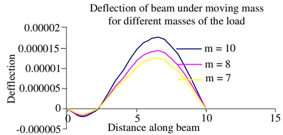
Fig. 2: Deflection of beam under moving mass for different masses of load
