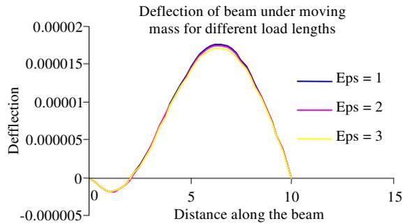
Fig. 3: Deflection of beam under moving mass for different load lengths
