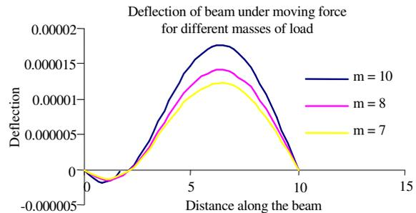
Fig. 4: Deflection of beam under moving force for different masses of load
