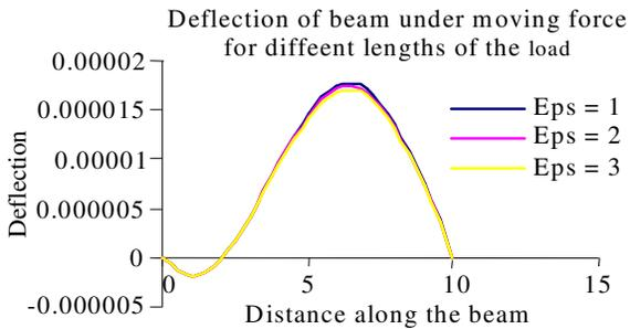
Fig. 5: Deflection of beam under moving force for different lengths of the load
