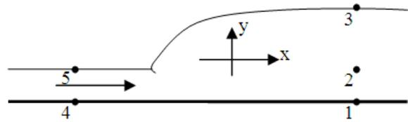
Fig. 1: Definition sketch of a hydraulic jump
