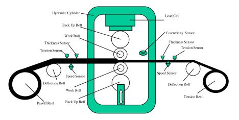
Fig. 1: The Reverse Rolling Mill
