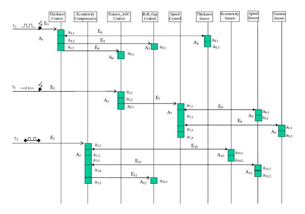
Table 1: Time Characteristics of Automatic Gauge Control System
